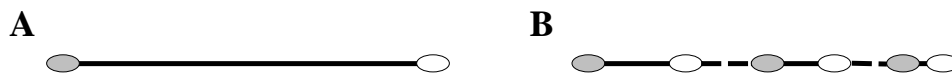
Figure 34: A) Ray traversing one pair of entry and exit points contains solid space. B) Ray traversing more than one pair of entry and exit points contains internal free spaces.
