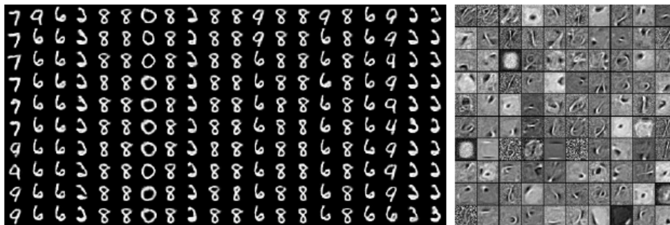
Figure 16.15: Samples from a trained RBM and its weights. ( Left ) Samples from a model trained on MNIST, drawn using Gibbs sampling. Each column is a separate Gibbs sampling process. Each row represents the output of another 1,000 steps of Gibbs sampling. Successive samples are highly correlated with one another. ( Right ) The corresponding weight vectors. Compare this to the samples and weights of a linear factor model, shown in figure 13.2. The samples here are much better because the RBM prior p(\mathbf{h}) is not constrained to be factorial. The RBM can learn which features should appear together when sampling. On the other hand, the RBM posterior p(\mathbf{h} | \mathbf{v}) is factorial, while the sparse coding posterior p(\mathbf{h} | \mathbf{v}) is not, so the sparse coding model may be better for feature extraction. Other models are able to have both a nonfactorial p(\mathbf{h}) and a nonfactorial p(\mathbf{h} | \mathbf{v}) . Image reproduced with permission from LISA (2008).
